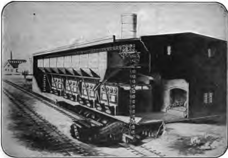
FIG. 99.—Power plant where mechanical devices carry coal from car to furnace, feed the furnace, and load the ashes on the cars.
